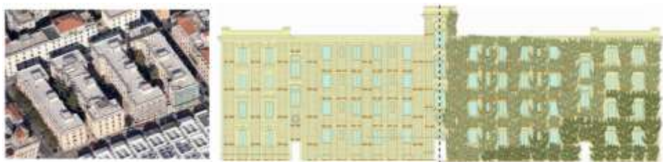
Figure 1: The picture of the case study block and the proposal for one of the courtyard façades. The bearing structure and the partition of the green wall: evergreen and deciduous plants in the lower and upper parts. (Sources: Google Maps, 2013; Results of the workshop 2013/14 by R. Di Berardino, L. Hernandez, P. Riccardi).
